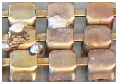
2 Too high temperature
