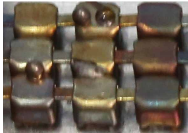
2 Too high temperature
