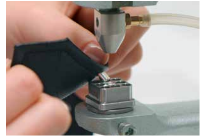
3 Turn the fabric around, place an already applied 3D Stud in one of the linear grid cavities, crystal side facing down.
