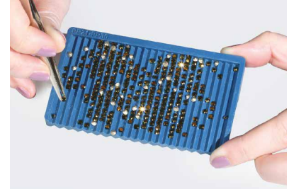
Using a Chaton Sieve can facilitate the setting of Chatons
