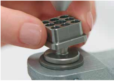
1 Position the linear grid on top of the lower die.
