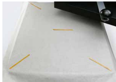
Test with temperature measuring strips (art. 9010/007)
